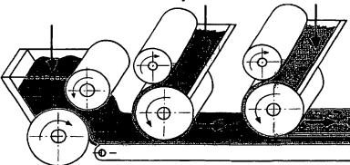
Conveyer belt to take layered slab through cooling tunnel and slitter
